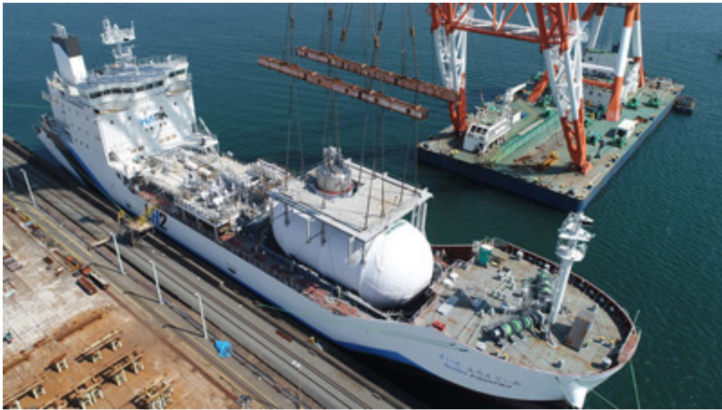
Figure 14 — World's first liquefied hydrogen carrier launched in Japan. Ce navire de 120m transportera 90t d'hydrogène 18
